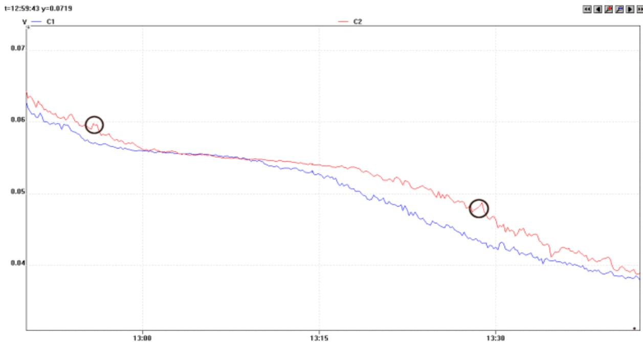
**Fig. 10 detail of capacitor discharge voltage under load**
