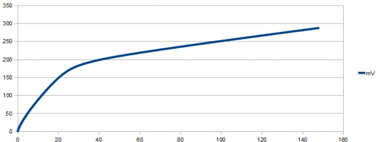
**Fig 1. 'spontaneous' voltage on capacitor vs. days since 1Mohm shunt removed**
