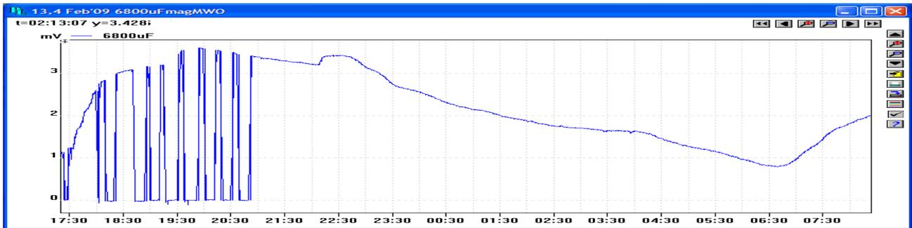
**Fig. 16 'spontaneous' voltage on capacitor inside Faraday cage**
